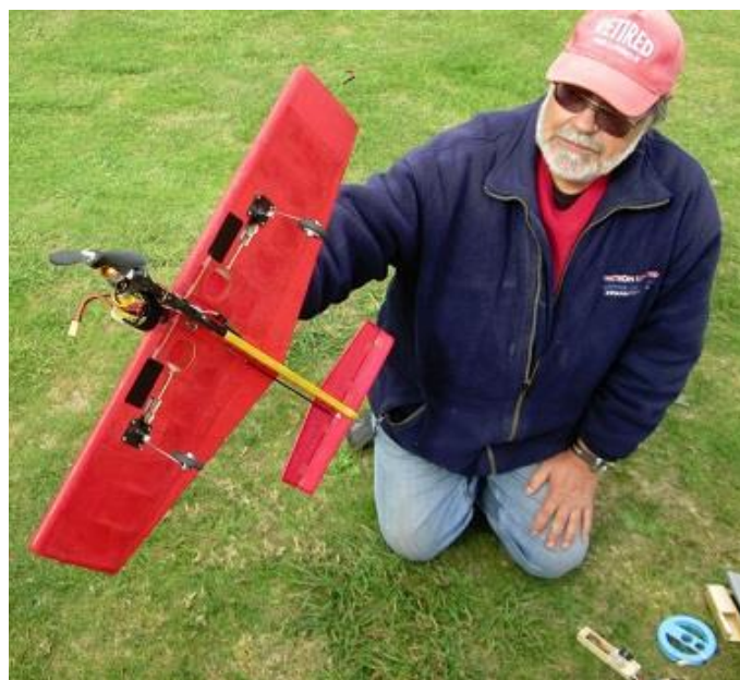
Den with control line proving airframe with retracts. 4 channel radio incorporated into handle as a removable module which can also be held separately, absolutely brilliant
