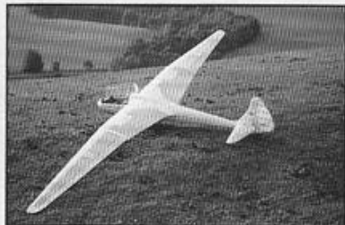
Long aileron on the outer panels make the model very scale-like in performance.
