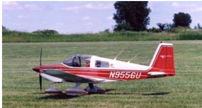
53. In take-off position at a grass field in Minnesota. Sturdy wheel pants work great on grass. 24-inch flying prop is same diameter as scale static prop.
