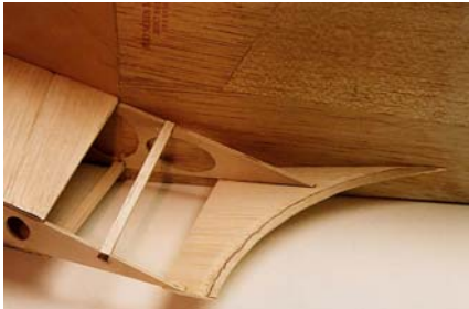
29. Rear wing filet is installed after joining front and rear fuselage halves. Tapered ply trailing edge.
