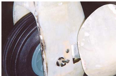
34. Outside of main pant shows threaded axle and two sheet metal screws. Speed fairing is being lowered in place to cover this stuff.
