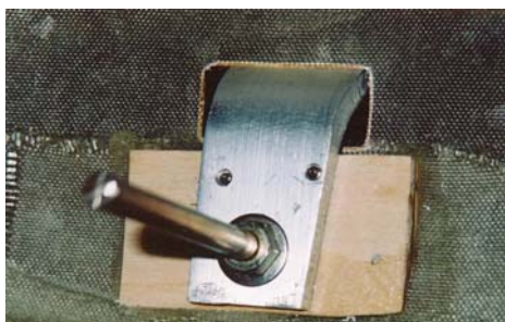
33. Main gear landing gear strut is bolted to inside of wheel pant with the axle and two sheet metal screws. Beveled ply epoxied to inside of pant distributes stress and provides flat surface for strut.
