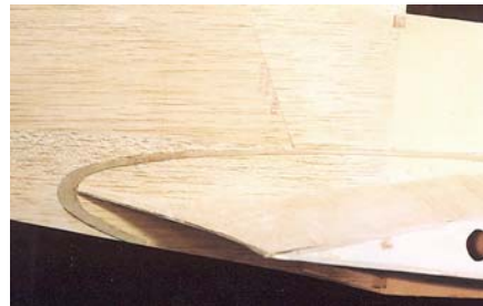
30. \frac{1}{64} " ply forms sheet-metal-like edge of wing filet.
