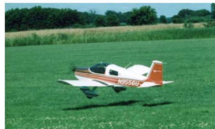
53. In take-off position at a grass field in Minnesota. Sturdy wheel pants work great on grass. 24-inch flying prop is same diameter as scale static prop.
