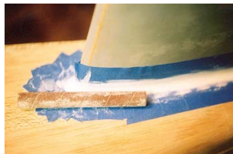
32. Stab filet is smoothed down to masking tape with a sanding spindle tube before removing masking tape.
