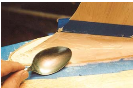
31. Epoxy and SIG microballoons mixture is applied to masked wing filet with a wet soup spoon.
