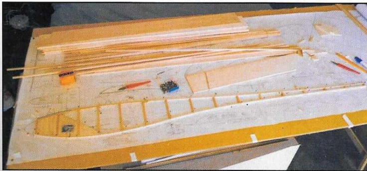
Left: scrap balsa supports are placed under the front of the ribs and front of trailing edge to keep profile correct. Split and re-cement leading edge at tips to curve.
