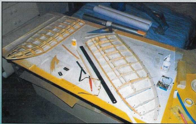
Left: scrap balsa supports are placed under the front of the ribs and front of trailing edge to keep profile correct. Split and re-cement leading edge at tips to curve.
