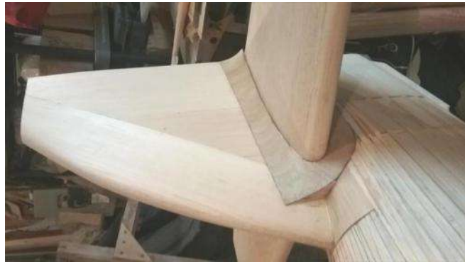
Install wing filets by same method. Alternatively, cut the stab filet from 1/64" ply. Pattern on plans.
