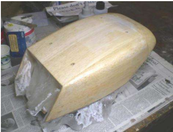
The entire radiator can be covered with one piece of \frac{3}{4} oz glass cloth.
