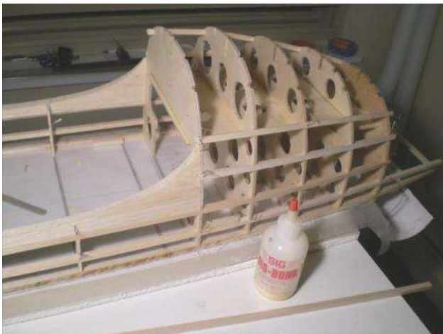
Add some stringers to the nose area to support the nose formers. Leave the bottom open for now.
