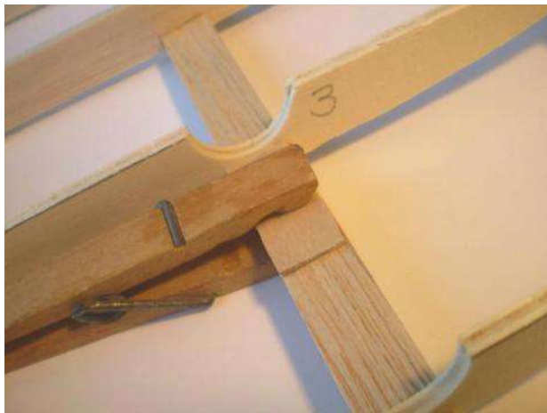
Add a ply patch to the lower spar where the bolts will be. Position the elevators over the stab's trailing edge spar. Mark the locations of the hinge extensions.
