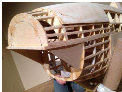
Inverted gas engine mounting, removable upper hatch. Enlarged firewall for 105CC inline twin Quadra 52.
