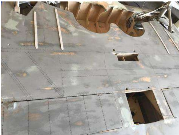
Add scale reinforcement strips and rivets on the bottom of the wing.
