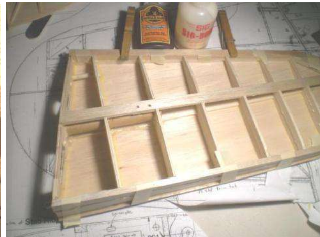
File a half hole at all hinge locations, top and bottom. Glue the upper and lower stab halves together. Add a 1/2" strip of 1/16" sheeting to the trailing edge of the lower half, leaving a 1/8" overhang as was done in the upper half. This will help alignment when fitting the elevators in the next step while leaving the interior accessible.
