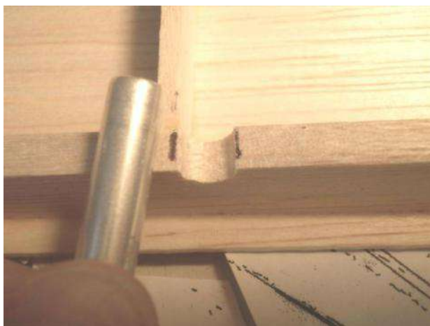
File a half hole at all hinge locations, top and bottom. Glue the upper and lower stab halves together. Add a 1/2" strip of 1/16" sheeting to the trailing edge of the lower half, leaving a 1/8" overhang as was done in the upper half. This will help alignment when fitting the elevators in the next step while leaving the interior accessible.
