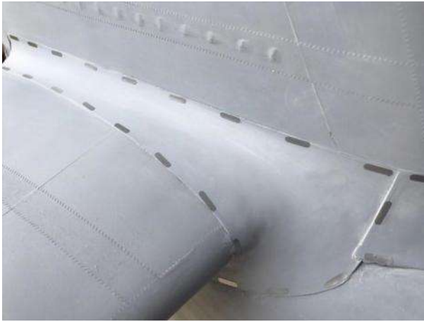
Rivet plates are vinyl stickers from Callie Graphics. Simulated Dzus fasteners.
