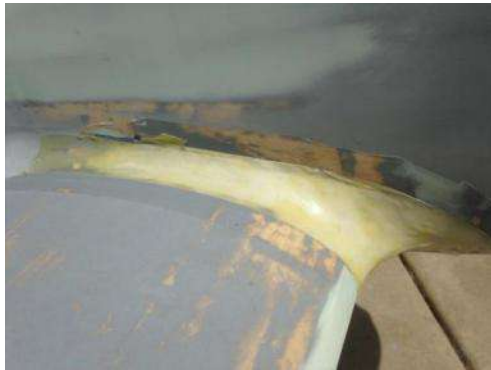
Install wing filets by same method. Alternatively, cut the stab filet from 1/64" ply. Pattern on plans.
