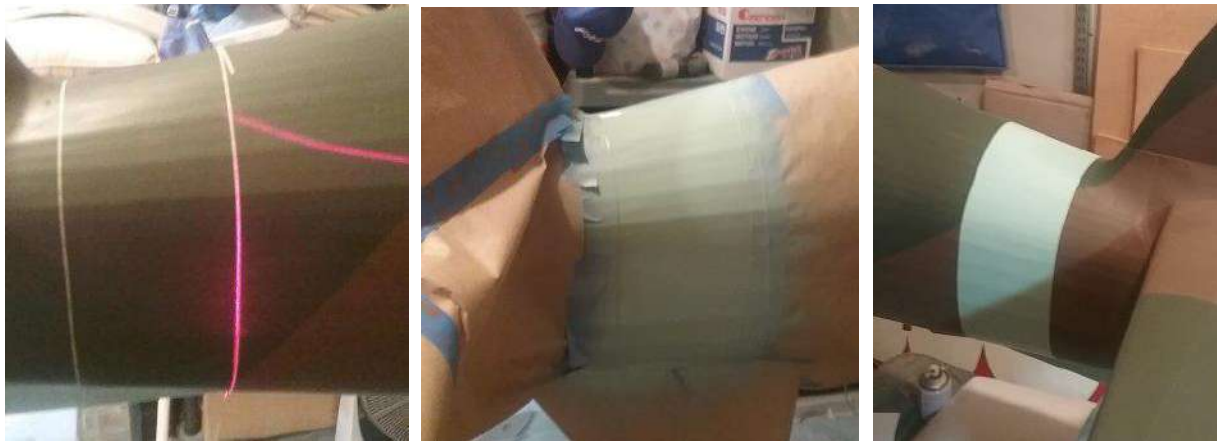
Draw invasion stripe with a carpenter's laser. Mask per laser line and spray.
