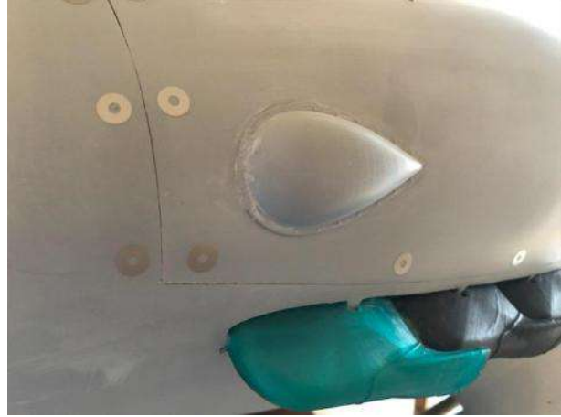
Rivet plates are vinyl stickers from Callie Graphics. Simulated Dzus fasteners.
