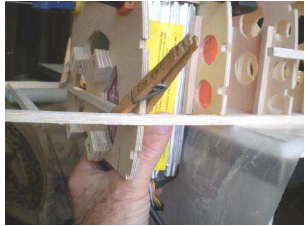
With crutch hanging over the edge, glue the firewall F3 in place. Before glue sets, trust but verify that the LiPo batteries will fit.
