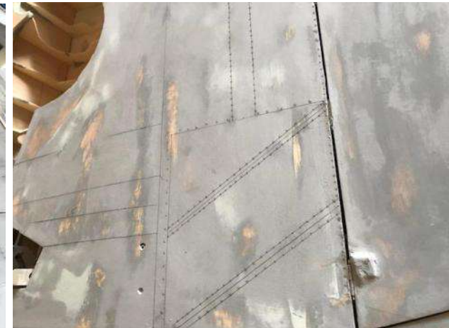
Add scale reinforcement strips and rivets on the bottom of the wing.
