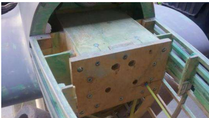
Inverted gas engine mounting, removable upper hatch. Enlarged firewall for 105CC inline twin Quadra 52.
