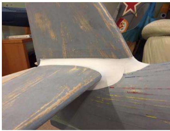
Light weight glass cloth is applied with epoxy resin. After curing, the excess is trimmed away with a razor blade.
