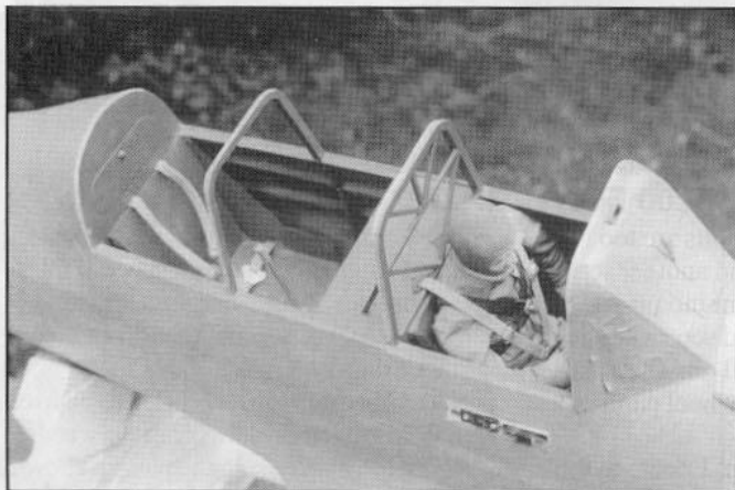
LEFT: Fuselage and windscreen are completed, ready for color paint before canopy is attached. RIGHT: Rough-cut canopy section clamped in place, marked for trimming. Rear to front installation.
