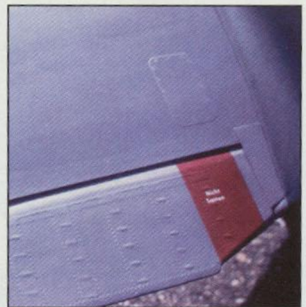
Glue-drop rib stitching on flap simulates fabric covering.
