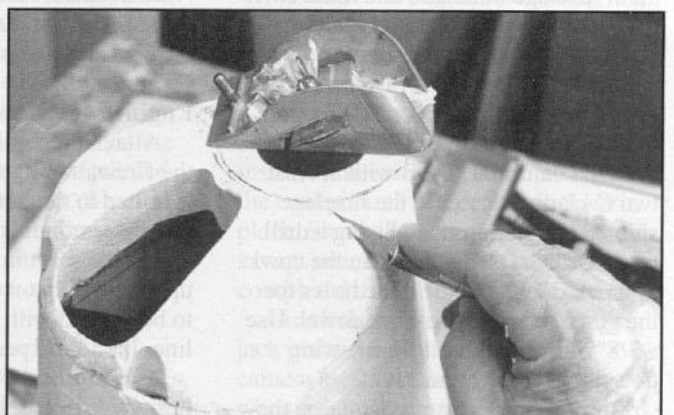
LEFT: Ply dummy exhaust pipe bracket epoxied in place inside cowl. RIGHT: Nose bowl being carved to shape with razor plane and X-Acto knife.
