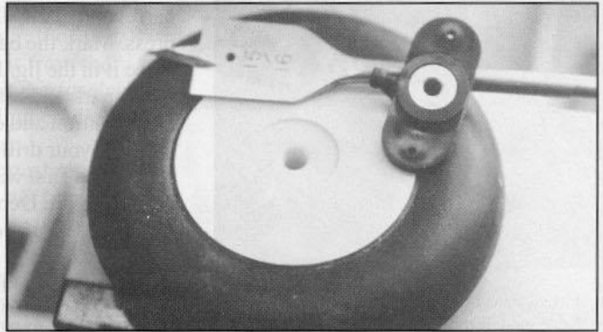
LEFT: Top surface is sheeted while wing is pinned to building board. Rear section left open for flap and aileron assembly. RIGHT: 1/32" deep recess is drilled in wheel hub for close fit of Sig wheel pant mount.
